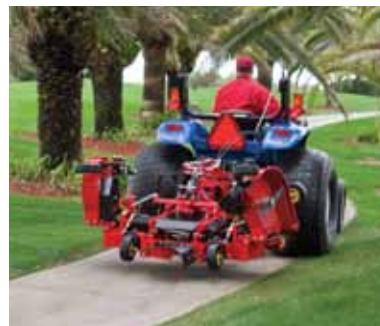
Outer two decks fold hydraulically to 78" (2 M) for transport
